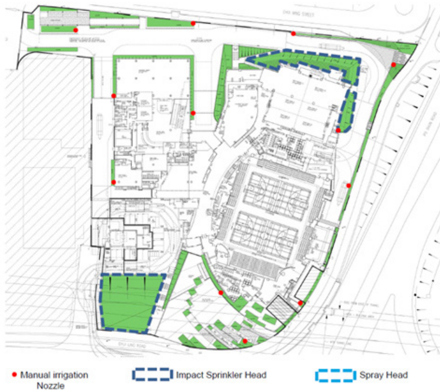
Figure 4 The layout of auto and manual irrigation
