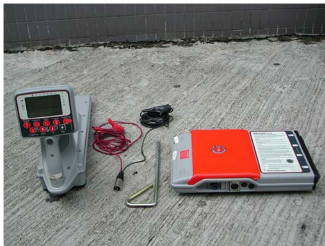
Plate C2 Components of Electromagnetic Type Detection Equipment
