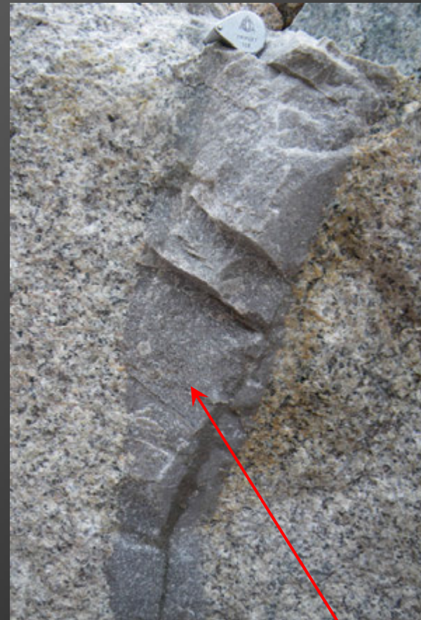
(b) A microcrystalline siliceous dyke (potentially alkali-reactive) in granite
