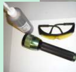
Use of Florescence Solution for Seepage Detection
