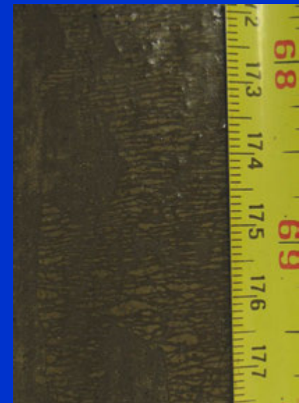
Multiple Cracking of Specimen
