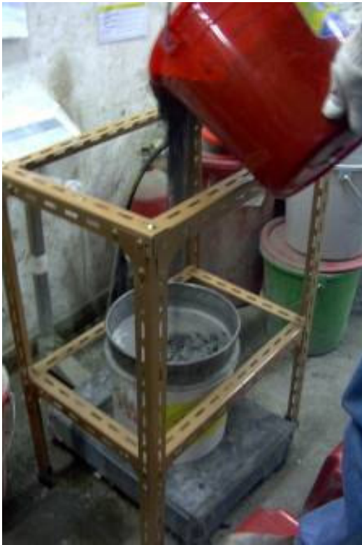
Step 2: Extract fine materials on the top layer by sieve
