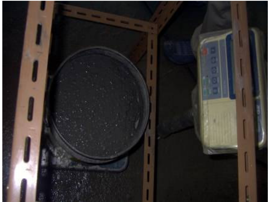
Step 3: Weight the percentage of fine materials
