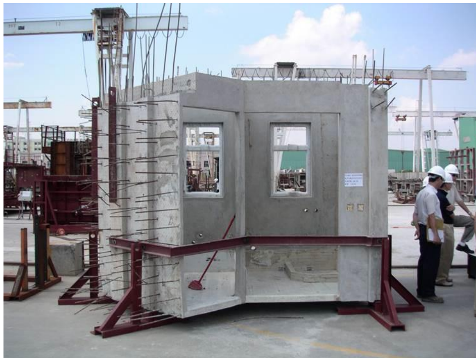
Photo 4 : Precast bathroom cum kitchen
