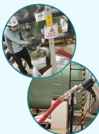
**The Portable Media Conveyor** is used for removing and refilling filter media in filter tanks, streamlining the material handling process while significantly reducing entry time to confined space, minimizing physical strain and the risk of injury.
