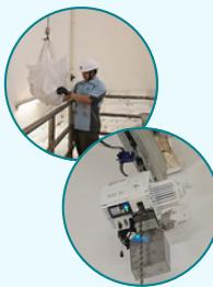
**The Moon Lifter** assists workers in lifting salt bags to the top of brine tank. It utilises real-time force and position detection to maintain dynamic balance, enabling smooth, stress-free movement, effectively achieving zero-weight maneuvering. Unlike traditional hoists, the Moon Lifter allows intuitive, hands-on control without the need for buttons, intelligently adjusting torque and speed in response to motion feedback for seamless and user-friendly operation.
