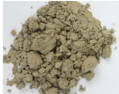
Primary Fly Ash, 50% cement replacement
