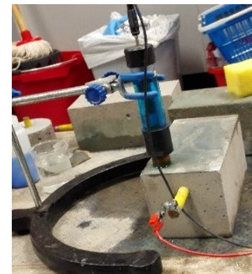
Half-cell potential measurement
