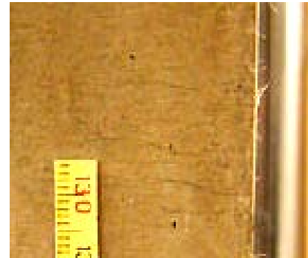
Multiple Cracks with Small Spacing and Opening in ECC
