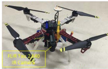
UAV-IR Integrated System (DJI F450)
