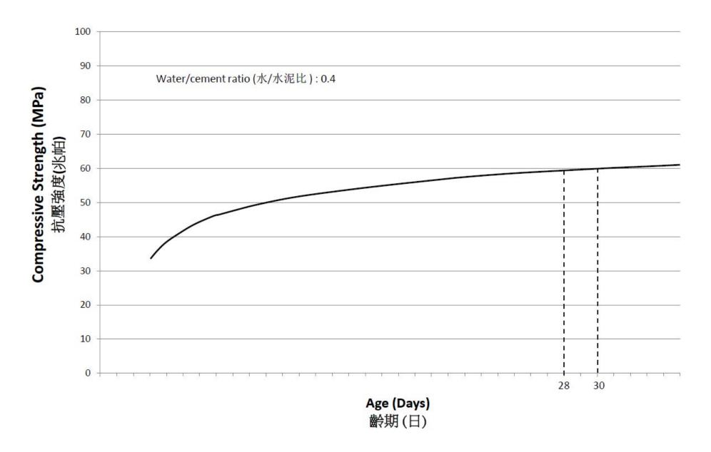
Extracted from A.M. Neville, *Properties of Concrete* (4th Edition), p304; with conversion to natural scale from log scale 節錄於A.M. Neville, *Properties of Concrete* (第四版), 304頁, 並將對數刻度轉成自然刻度
