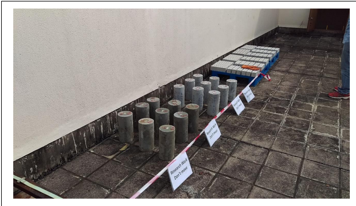
Figure 7.1 Cylinder Specimens Stored on the Rooftop of PWCL Building
