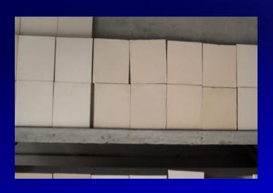
Mock-up/Control samples with varying levels of colour/acid etching/ tooling etc
