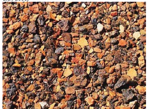
Inorganic growing medium in Stuttgart, made from recycled construction and industrial waste, including crushed clay tiles and steel mill slag. (Source: Urbis Ltd)
