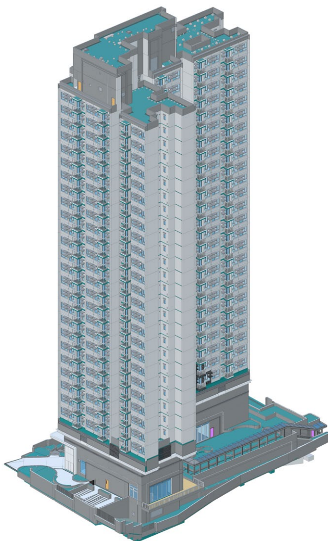
HKHS's Hung Shui Kiu/ Ha Tsuen New Development Area Dedicated Rehousing Estate Project Phase IA with GBPs generated by BIM models.
