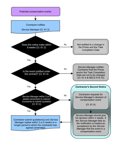
B6.3.2.11 A process map showing the procedures in notifying compensation event is shown in the diagram below:
